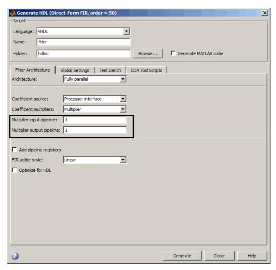
The coder enables the **Multiplier input pipeline** and **Multiplier output pipeline** options when **Coefficient multipliers** is set to Multiplier.
