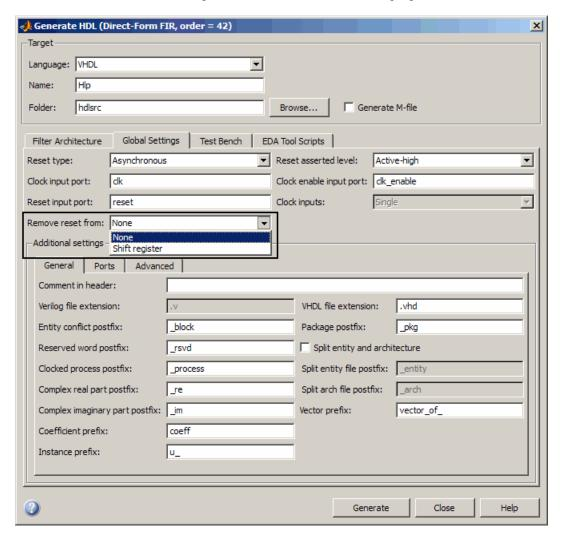
You can also use <code>generatehdl</code> function with the property <code>RemoveResetFrom</code> to suppress generation of resets from shift registers.
